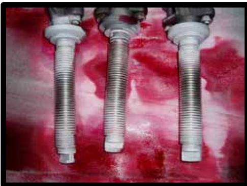
Post cycling penetrant test of bellows
