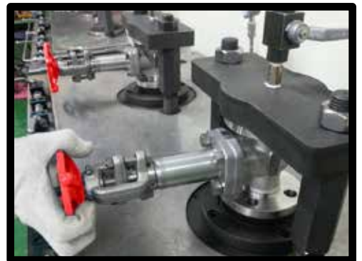
Pressure testing of each valve
